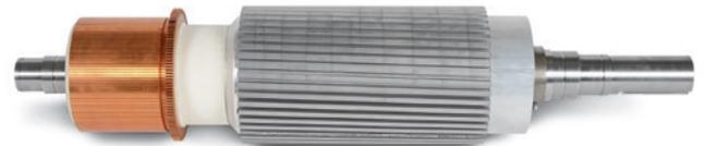
▲ Placement of the coils within the core slots and the precise slot skew allows for higher torque and improved commutating as compared to older DC motor technologies.
